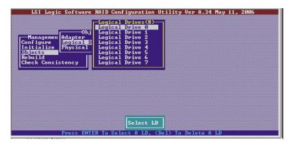
Figure 3-3: Logical Drive Submenu
